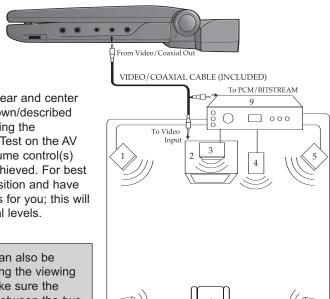
Place the subwoofer, front, rear and center speakers in locations as shown/described here. After correctly positioning the speakers, perform the Tone Test on the AV Amplifier and adjust the Volume control(s) until the desired sound is achieved. For best results, sit in the viewing position and have someone adjust the volumes for you; this will enable you to set the optimal levels.
